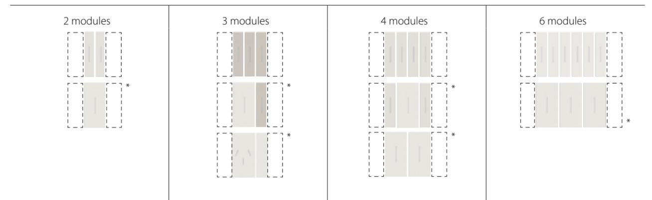
\* Note: for solutions using one 2-module cover for the main controls, it will be necessary to use two "half-module blanking modules" (item K4949) at the sides of the control. (see the sample diagrams below)
