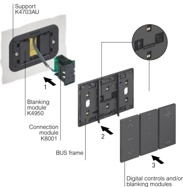
At the side of the connection module, install 2 blanking modules, item K4950, in any position.
