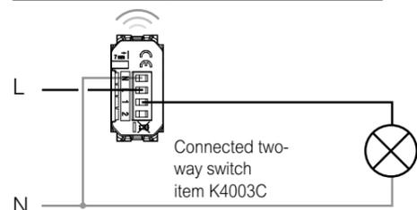
Wiring diagram - redirected or inverted
