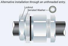
If the apparatus is untapped use a locknut.
