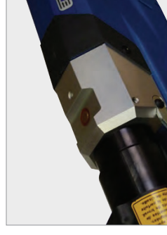
Visual Crimp Indicator - Audible Click & Visual Indicator
