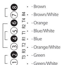
T568A Cabling Pinout Specifications
