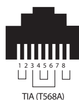
T568A Cabling Pinout Specifications
