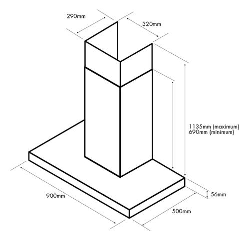
**IMPORTANT** These dimensions are a guide only. All measurements are in millimetres (mm). For complete installation instructions, refer to the manual provided with product.
