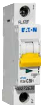
MCB 10 kA, trip curve C: rated current up to 63 A, rated breaking capacity 10 kA to IEC/EN 60898
