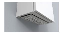
**Description:** The rubber grommet is very simple to use. The installation does not require tools, which in turn means lower work cost. The "pushout" membrane is a permanent seal until it is penetrated by a cable or pipe. Suitable for holes in materials of 0.5 to 4 mm thickness.
