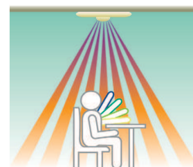
Quad element sensor to detect a small hand waving movement
