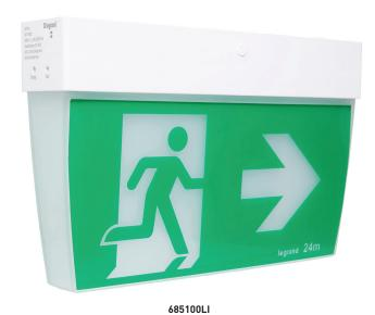
**Specifications** Mode of operation Maintained Supply voltage 240V a.c. +/- 6% 50Hz 3.5W Power consumption **Battery** Li-ion 6.4V 570mAh Operating temperature 10° to 40° IP rating IP20 **Body construction** Polycarbonate Diffuser construction Polycarbonate AS/NZS 2293 AS/NZS60598 🔬 🔔 Compliance
