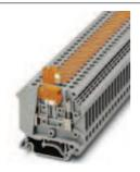
Knife disconnect terminal block, Connection type: Screw connection, Cross section: 0.2 mm² - 4 mm², AWG: 24 - 12, Nominal current: 16 A, Nominal voltage: 500 V, Length: 51 mm, Width: 6.2 mm, Color: blue, Assembly: NS 32, NS 35/7,5, NS 35/15
