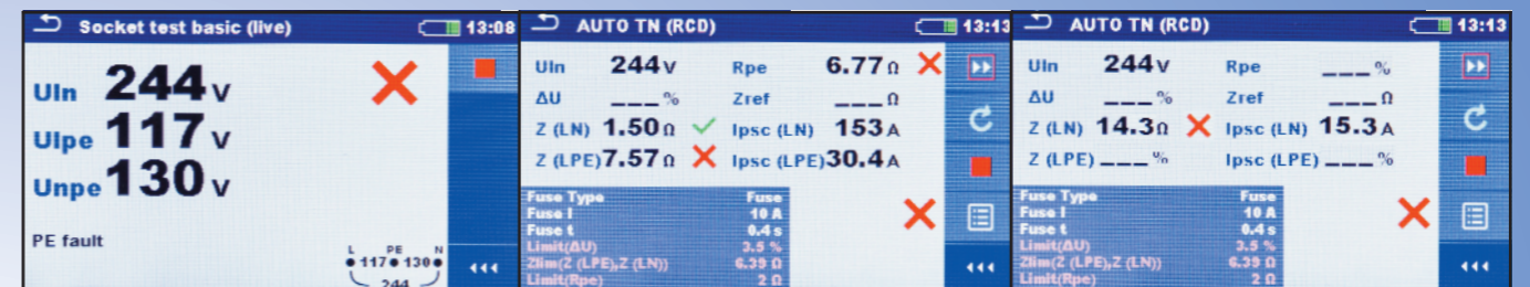
Earth Open Circuit FAIL Result Earth 6 Ohm FAIL Result Neutral-Earth Reversal FAIL Result
