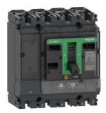
Circuit breaker, ComPacT NSX160F, 36kA/415VAC, 4 poles 3D (neutral not protected), TMD trip unit 125A
