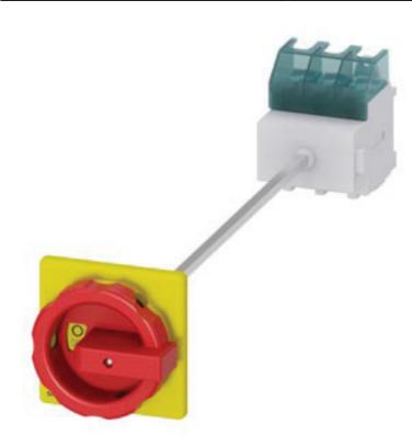
EMERG. STOP SWITCH 3-POLE IU=63, P/AC-23A AT 400V=22KW FLOOR MOUNTING DIN RAIL/TWO-HOLE MOUNTING ROTARY ACTUATOR RED/YELLOW (EMERG. STOP)
