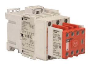
Safety Contactor 3 pole 43A 22KW 1N/O 4N/C auxiliary 110V AC Coil
