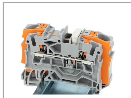
Step-down jumper (2006-499) commons 6 / 4 mm 2 (10/12 AWG) terminal blocks (2206 / 2204 Series) with 4/2.5/1.5 mm 2 (12/14/16 AWG) terminal blocks (2204/2202/2201 Series).
