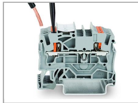
Insert fine-stranded conductors via operating tool.
