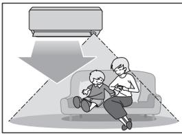
The air conditioner is in normal operation while the sensor is detecting human movement.
