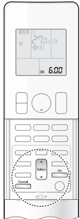
Timer functions are useful for automatically switching the air conditioner on or off at night or in the morning. You can also use the ON TIMER and OFF TIMER together.
