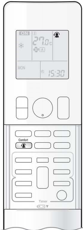
**COMFORT AIRFLOW operation:** The flow of air will be in the upward direction while in COOL operation and in the downward direction while in HEAT operation, which will provide a comfortable wind that will not come in direct contact with people.
