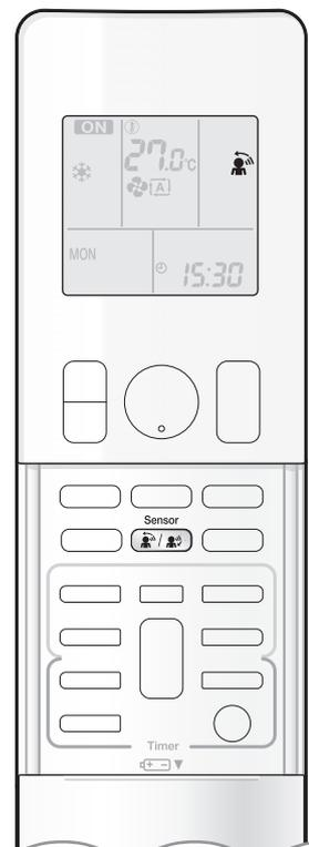
The INTELLIGENT EYE operation detects human movement and adjusts airflow direction. It can be set to avoid people or to direct airflow specifically at people. If no one is detected in the room for more than 20 minutes, the unit automatically enters energy saving operation.
