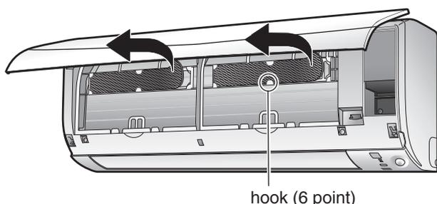
**3. Clean or replace the titanium apatite photocatalytic air-purifying filters.**
