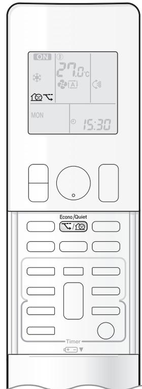
**ECONO operation** enables efficient operation by limiting the maximum power consumption.
