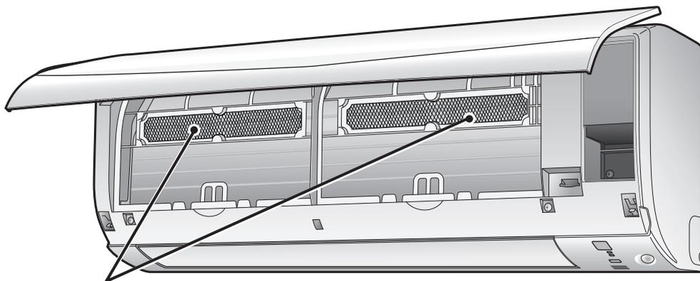
Titanium apatite photocatalytic air-purifying filter
