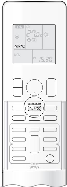
ECONO operation enables efficient operation by limiting the maximum power consumption. This function is useful to prevent the circuit breaker from tripping when the unit operates alongside other appliances on the same circuit.
